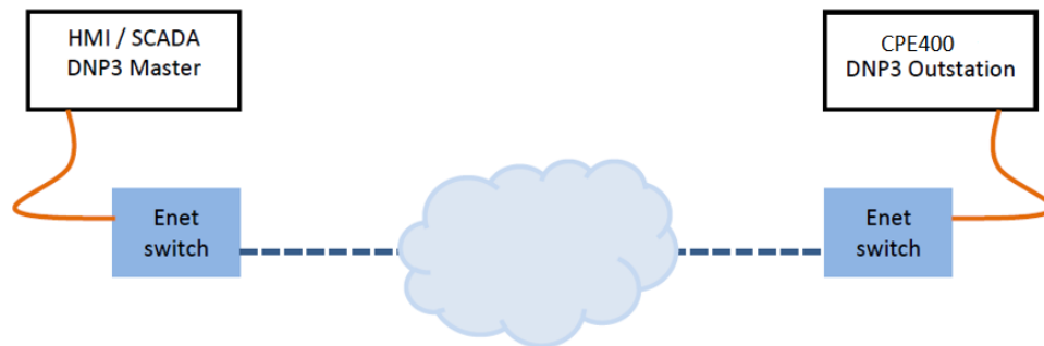
Figure 1: DNP3 Basic System Architecture
